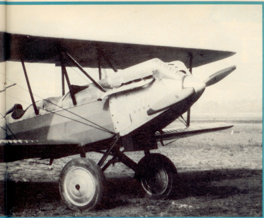
In 1929 the LP-3 was updated by rearranging the center struts and enlarging the vertical fin. The LP-3 here retained the OX-5 engine, but the LP-3A's used a Wright-Hispano.
