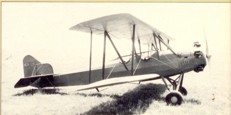
The final Lincoln-Page product was the Page Trainer, a two-seat trainer derived from the LP-3. The PT-K model, shown here was identical to the PT-W model except for the engine.
